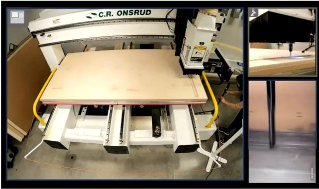
Figure 4. Multiple cameras capturing CNC router operation. Author.
